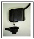
2. Remove magnetic impeller from motor cavity and rinse both under sink to remove slime build-up and any debris.
