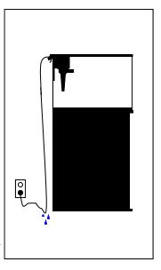
unplug the cord. Disconnect the fuse to the circuit breaker that supplies power to the appliance. Then unplug and examine for the presence of water in the receptacle.
